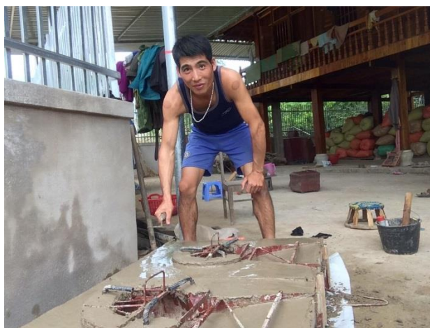
Picture 1: Producing improved cookstove by villager
