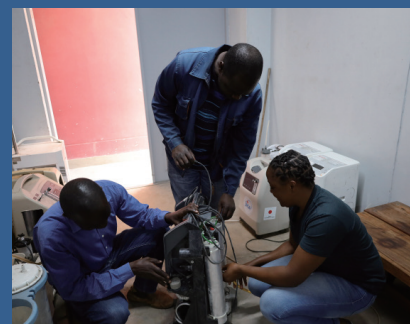
Mr. Darius and the Bio medical Technologist team repairing an Oxygen Concentrator
