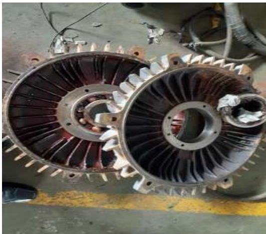
The front cover of motor full of leaves and sliver
