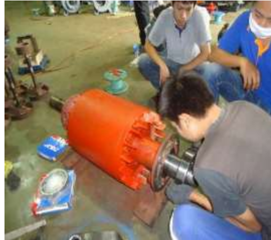
Put bearing into the shaft
