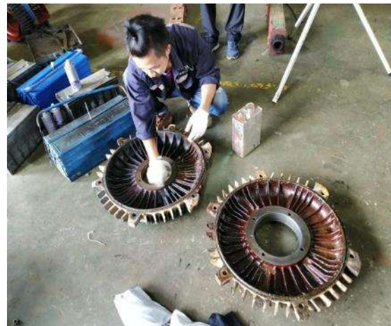
The front cover of motor full of leaves and sliver
