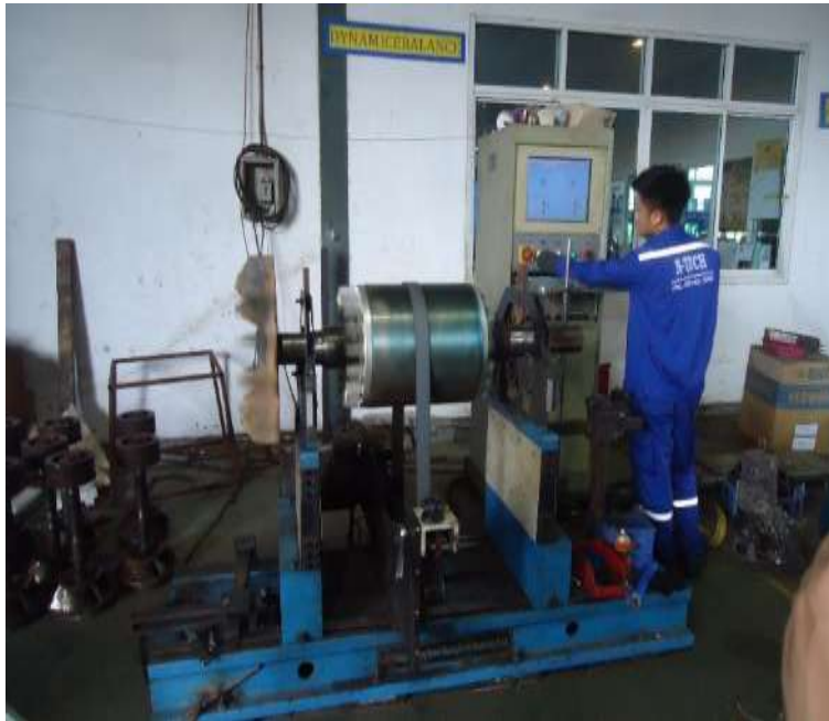
Balancing the motor
