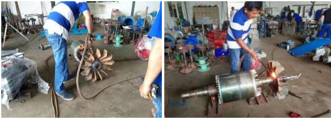
Burning the propeller hole
