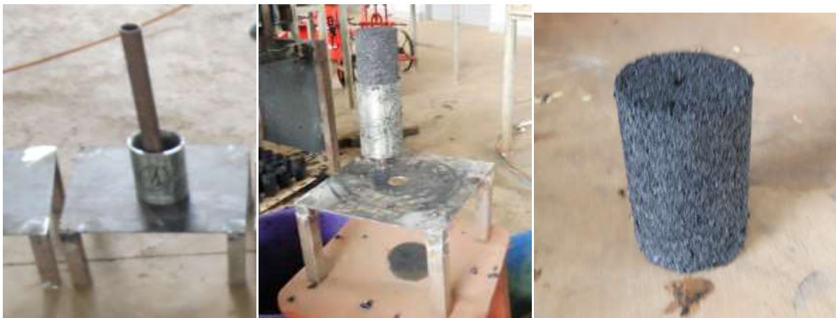
Demonstration of rice husk charcoal briquettest using with Manual Pressing capasitas one briquettes per process in Antsirabe
