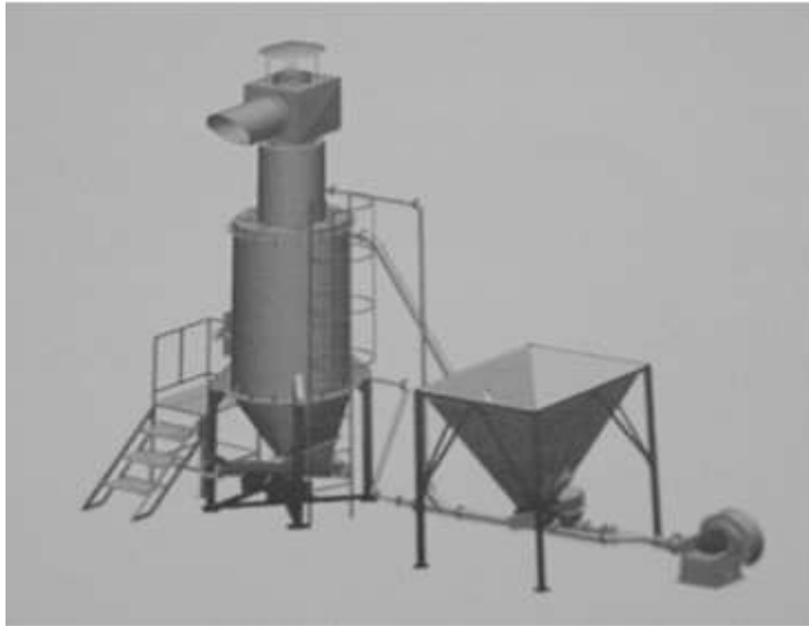
Figure 25. Cyclonic Husk Furnace Type AHF-250C made in Indonesia
