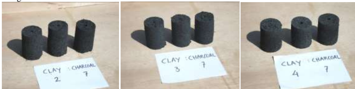
Figure 34. Concentration of glue and rice husk charcoal used produce charcoal briquettes
