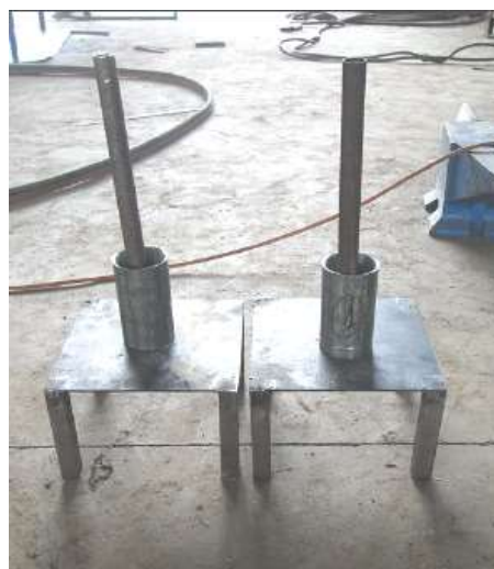
Figure 29. Prototype 1A of Pressing machine for charcoal briquettes
