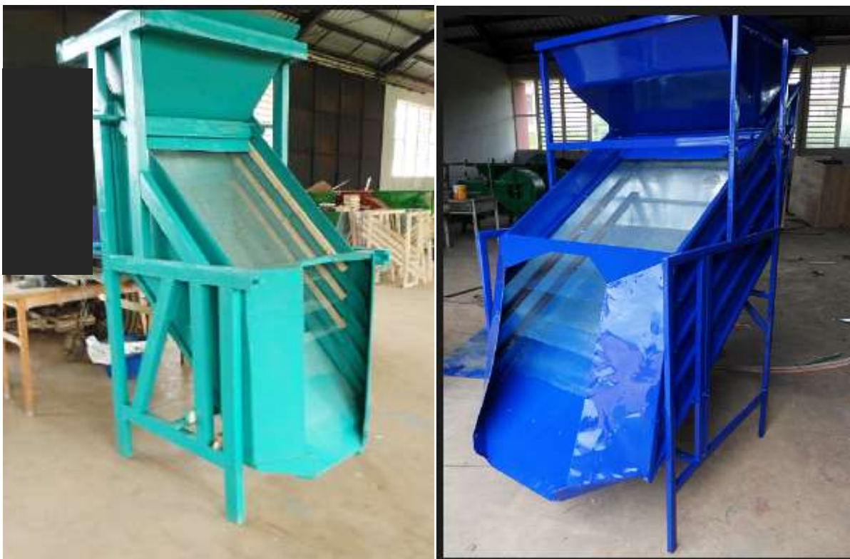
Figure 27. Prototype of Manual Paddy Separator from wood (1) and metal (2)
