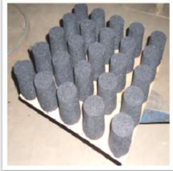
Figure 38. Demonstration of rice husk charcoal briquettest using with Manual Pressing capasitas 25 briquettes per process in Antsirabe
