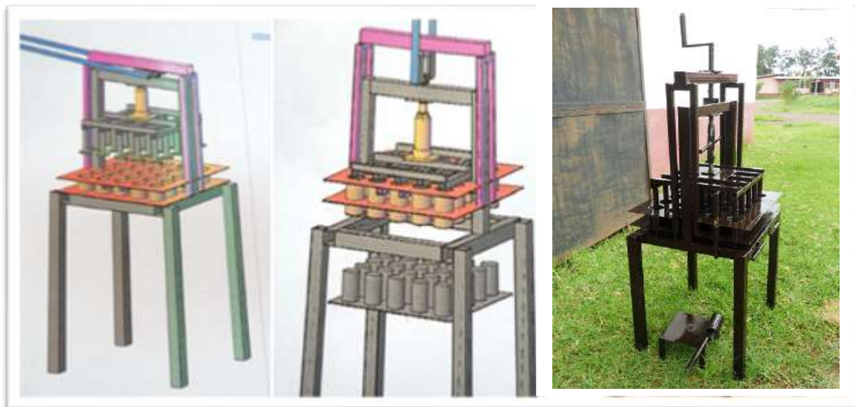
Figure 30. Prototype 1B of Pressing machine for charcoal briquettes
