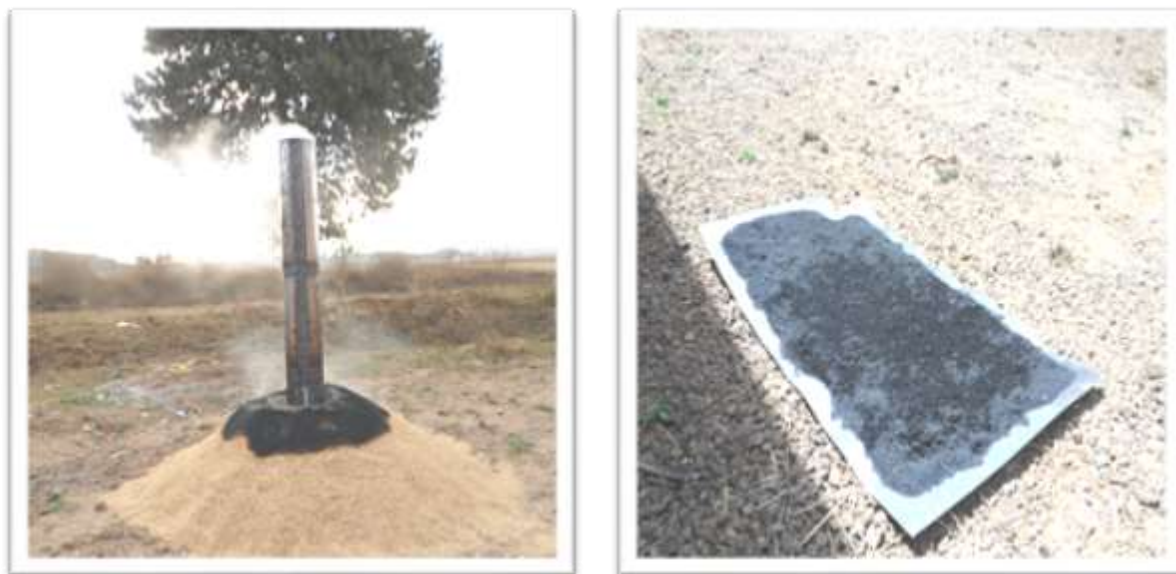
Figure 32. Test of rice husk charcoal burner
