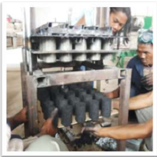
Figure 38. Demonstration of rice husk charcoal briquettest using with Manual Pressing capasitas 25 briquettes per process in Antsirabe
