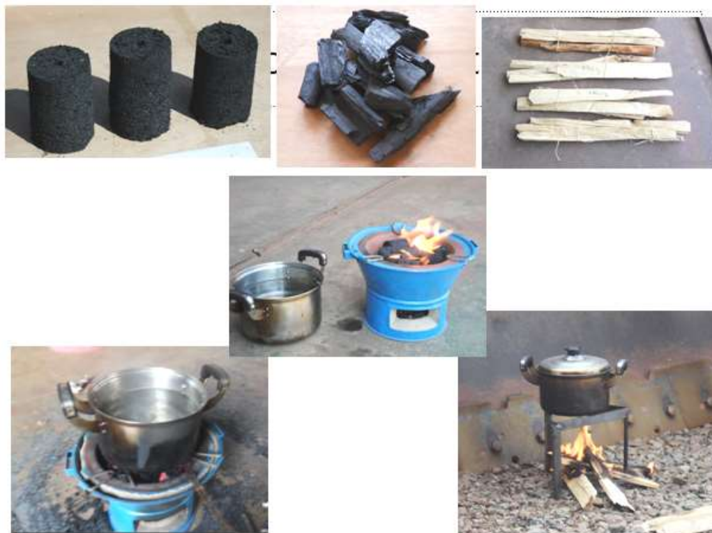
Figure 35. Test of rice husk charcoal briquettes and cost of energy for water cooking of 2 liters
