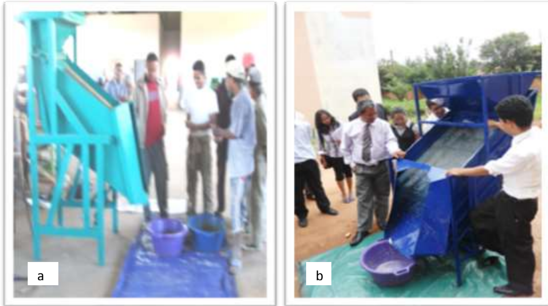
Figure 36 . Demonstration of new prototype Paddy Separator (a) material wood and (b) material metal in the CFAMA and Rice Milling, Antsirabe
