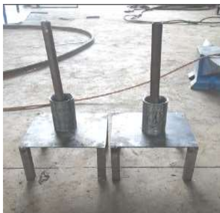
Figure 36. Prototype of Press machine for the rice husk charcoal briquettes model A2.
