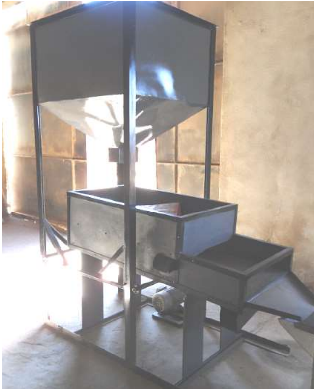
Figure 32. Prototype of paddy cleaner
