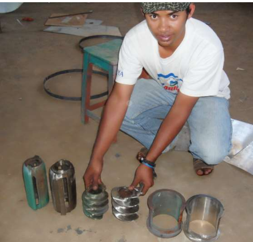
To change the spare part of rice milling unit (RMU) with metal material to stainless steel
