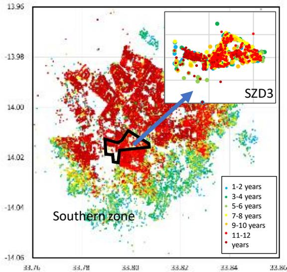
Fig.12 Distribution of water meter installation years in the Southern Zone and pilot DMA
