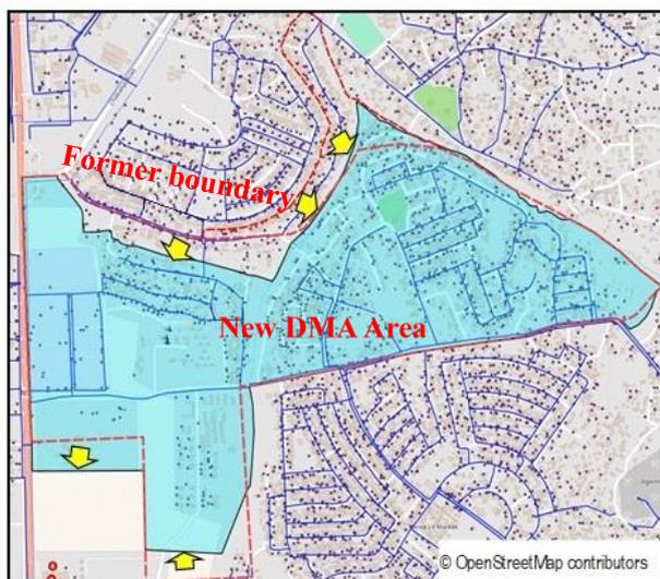
Fig.10 Reset of DMA boundary
