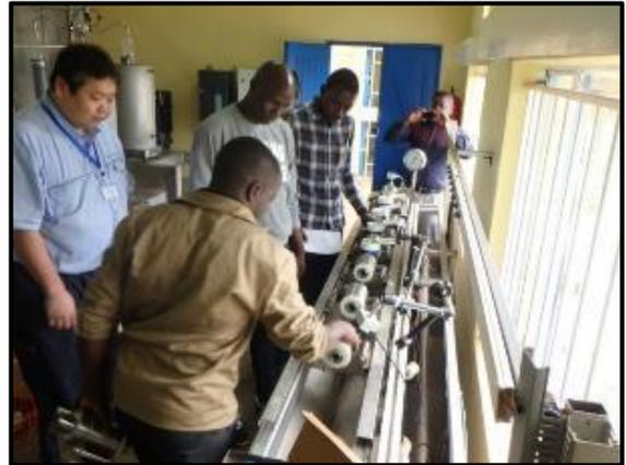
Photo 2: LWB proprietary water meter accuracy test
