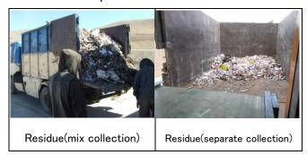
The amount of valuables shows about 10% is for mix collection waste and about 50 % is for separate collection waste. The amounts of RPF materials are 2.9%, 5.8%, 26.9%, 30.4% shown in the table from left to right. Therefore, technically speaking, separate collection is more desirable than mix collection and belt conveyor sorting is more desirable than hand sorting in terms of collecting RPF materials.
