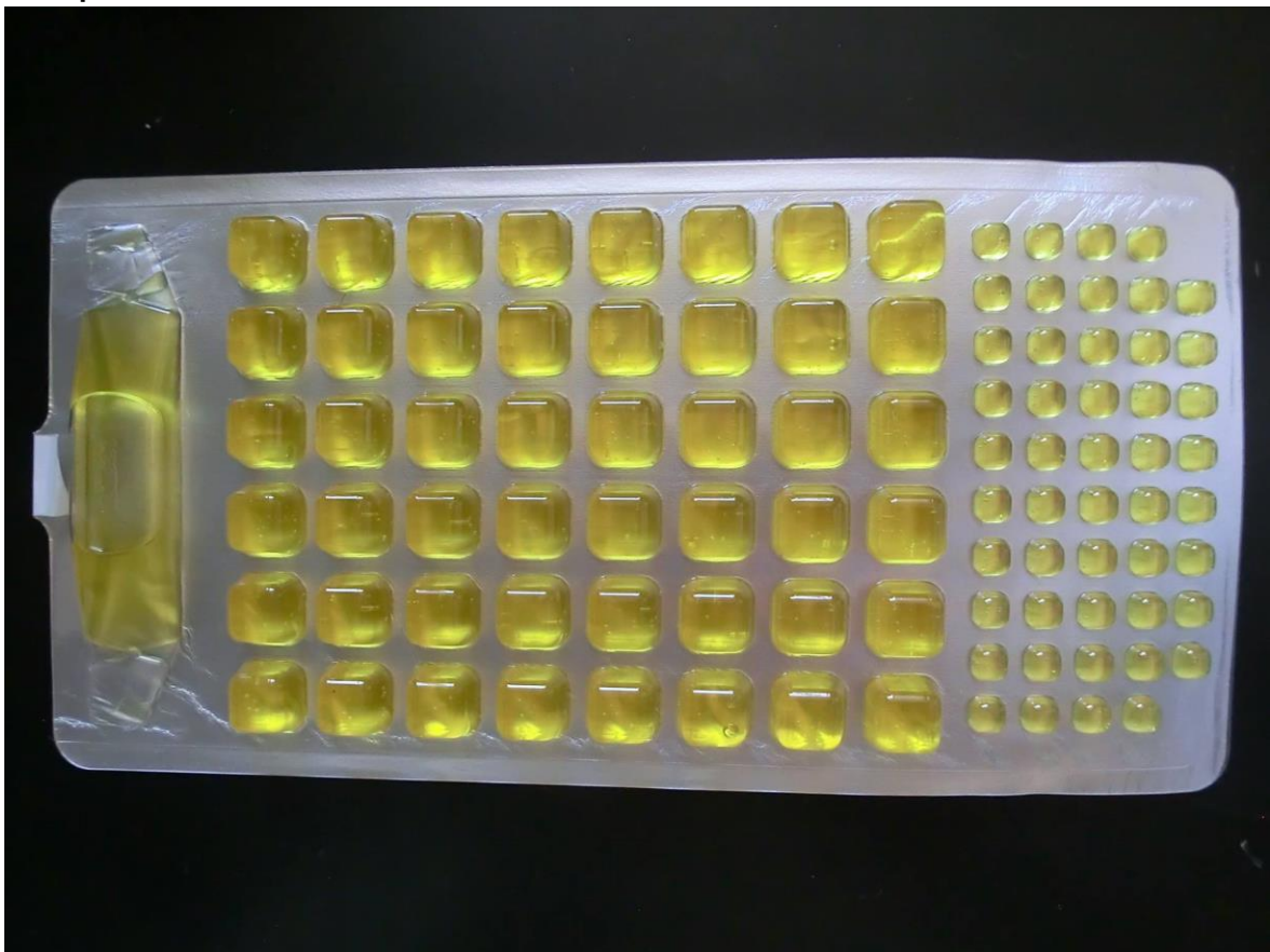
Figure 3. Yellow discoloration showing presence of total coliform.
