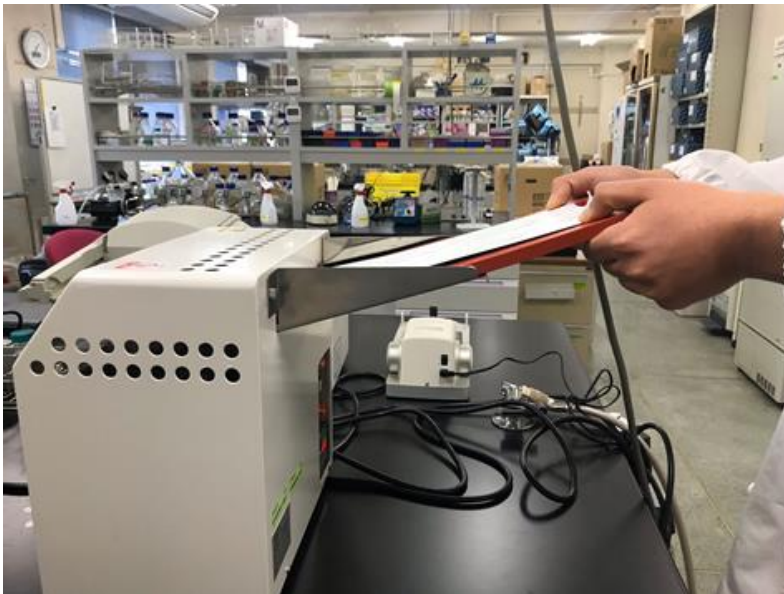
Figure 2. Sealing of Quanti- tray once the sealer has attained the temperature of 180^{\circ}\text{C} .
