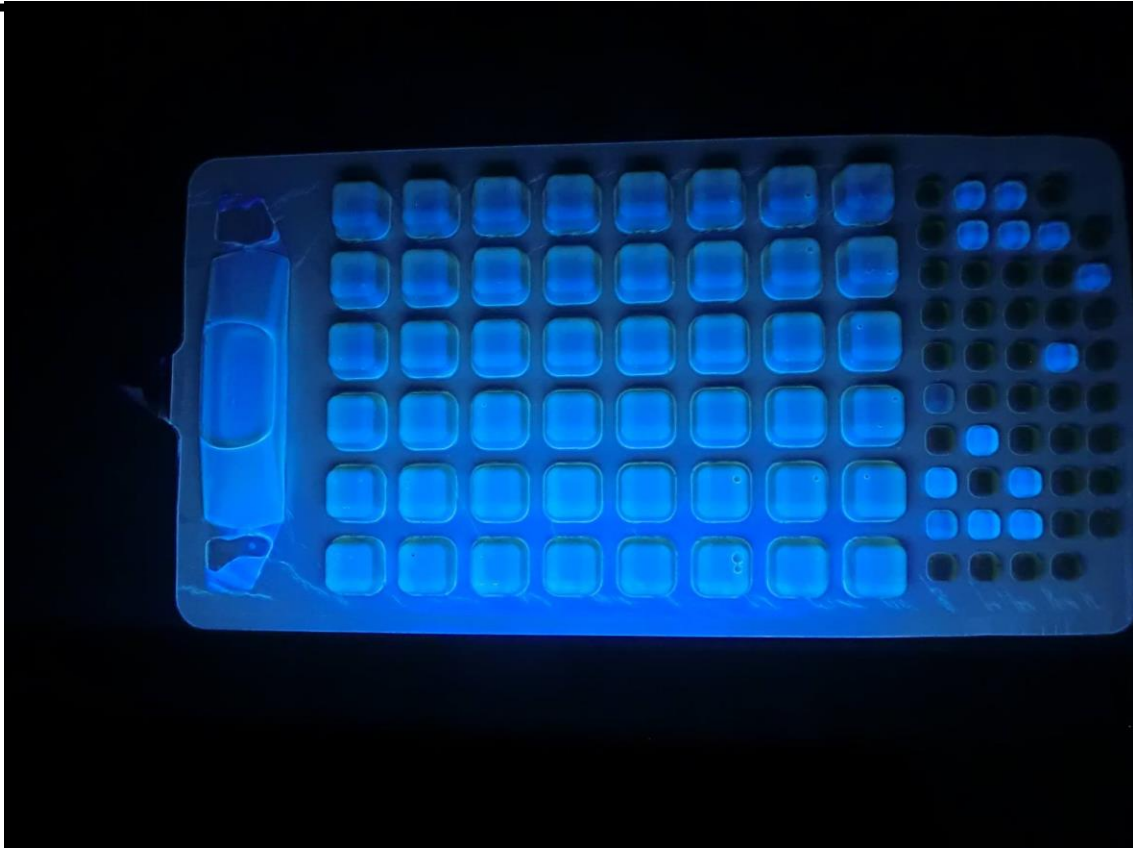
Figure 4. Fluorescent wells showing presence of E. coli
