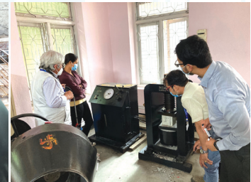
Compressive Strength Test of Concrete
