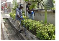
Microphone Leak Detector
