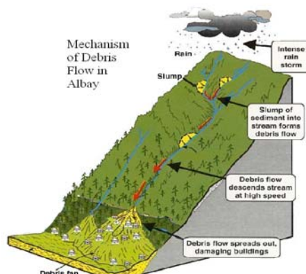
Mechanism of Debris Flow Schematic diagram of mechanism of debris flow that triggered numerous debris flows in Mayon
