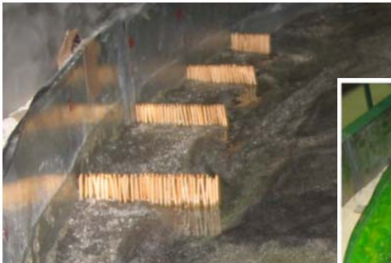
Figure 8, Permeable Type Spur Dike Model
