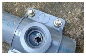
Photo 2 Drilled hole with burr
