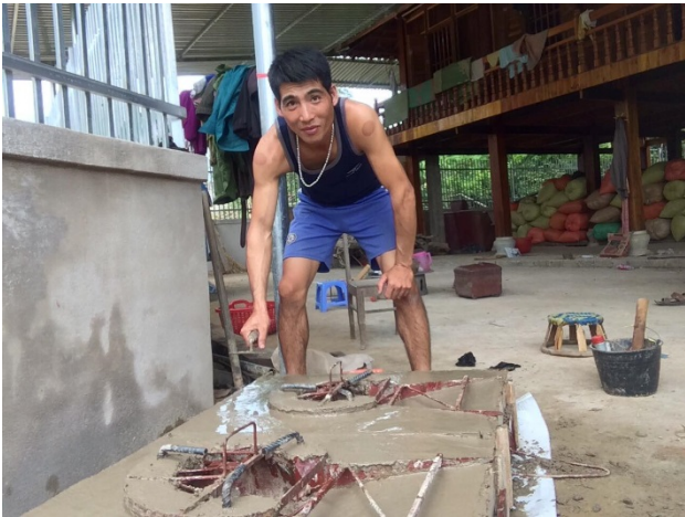
Picture 1: Producing improved cookstove by villager
