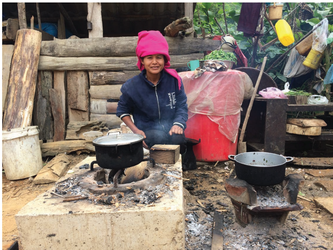
New ICS for cooking in Dien Bien (the cooking stove on the right side of picture is an older style of Lao cooking stove)
