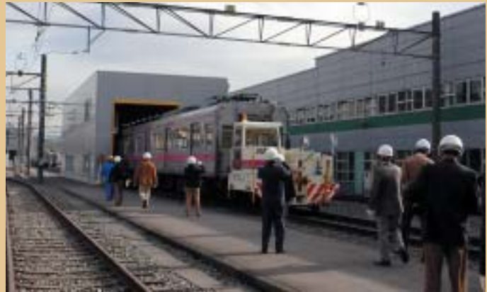
▲ This is the washing system for components under the railcar floor. It takes fifteen minutes to wash a railcar and uses only hot water of 60 degrees centigrade with no detergent, not to damage the electrical equipment.
