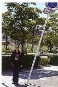
Meltem with a signpost inclined due to the soil liquefaction
